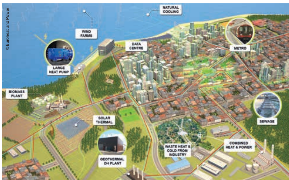
District heating is supplied from a variety of sources: solar and wind systems, waste incineration, biomass, geothermal energy, and industrial waste heat
