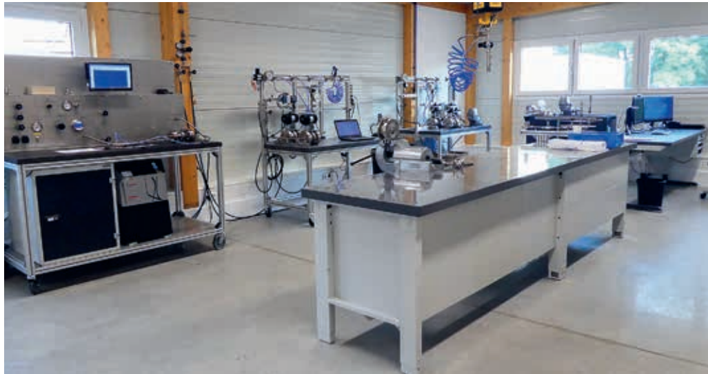
We would like to introduce our newest test benches from left to right: leak tightness test bench, life cycle test bench, torque behavior test bench, and the analysis station.
